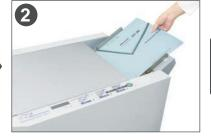
Insert prints, align the side guide, then press the start button. The booklets are produced immediately.
