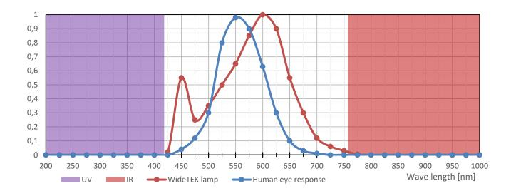
The radiated spectrum of the LED light on a WideTEK or Bookeye scanner is between 420 and 760 nm. This is completely inside the visible spectrum of the human eye. There is no emission of UV light (pink area at the left side of the diagram) and no emission of IR (red area at the right side of the diagram), only useful light is emitted (middle section).
