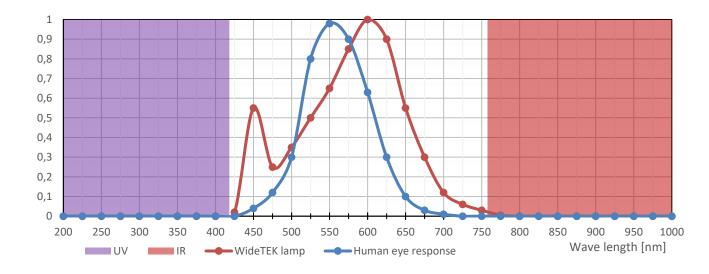
The radiated spectrum of the LED light on a WideTEK ART is between 420 and 760 nm. This is completely inside the visible spectrum of the human eye. There is no emission of UV light (pink area at the left side of the diagram) and no emission of IR (red area at the right side of the diagram), only useful light is emitted (middle section).
